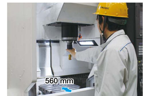
Machine front to table center 560 mm
